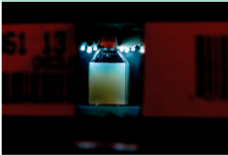
Photo of 30-ml flask viewed through an easy access “window” opening in a growth chamber created from a shoebox and white LED holiday lights.
