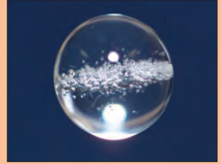
A water drop spun off during a microgravity crystallization experiment takes on a spherical shape. Without buoyancy, gas bubbles do not rise, but remain inside the drop.
