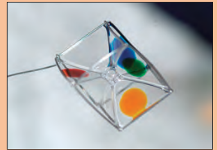
View of surface tension demonstration in microgravity using water being held in place by a metal loop. Drops of food coloring are for demonstration only.
