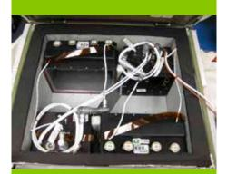
Top view, inside a CGBA insert housing small spider habitats (upper left and lower right) and cameras, part of Mission STS-134. Photo courtesy of BioServe Space Technologies.
