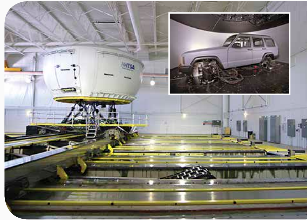
This is the high-bay area that houses the NADS simulator. The Jeep Cherokee module is inside of the white structure in the air—NADS is huge!
