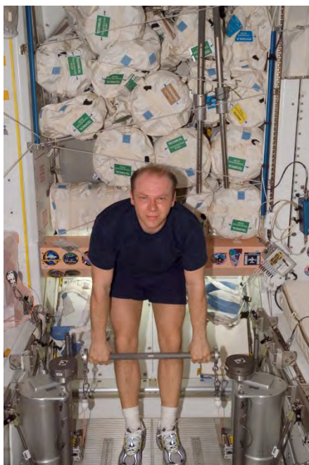
Cosmonaut Oleg V. Kotov works out on the Interim Resistance Exercise Device on the International Space Station. Mechanisms in the two adjustable mechanisms in the cylinders to Kotov's right and left provide lift resistance to the bar.
