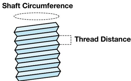
$$\text{Screw MA} = \frac{\text{Circumference of screw shaft}}{\text{Distance between threads}}$$
