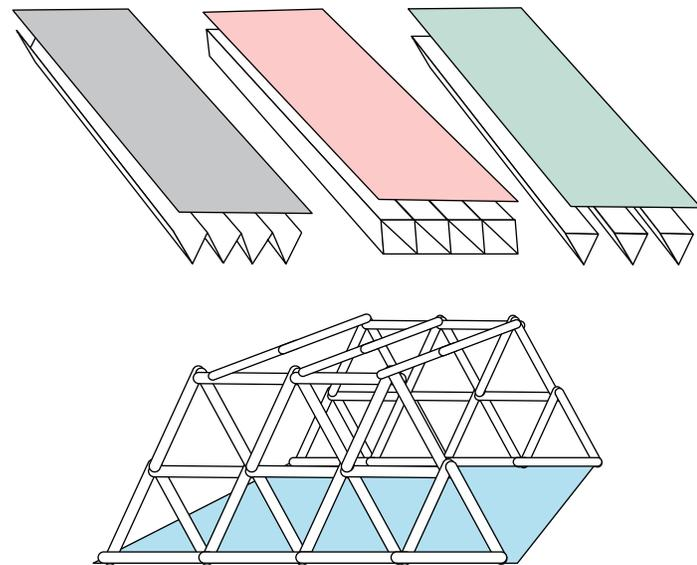
A successful bridge can be made from just two file folders and masking tape. If desired, additional supplies can be made available for construction such as craft sticks, drinking straws, toothpicks, and white glue.
