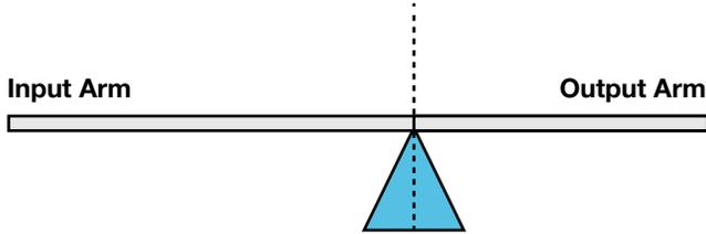
$$\text{Lever MA} = \frac{\text{Length of the input arm}}{\text{Length of the output arm}}$$
