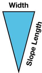
$$\text{Wedge MA} = \frac{\text{Length of slope}}{\text{Width of the wedge}}$$
