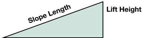
$$\text{Inclined Plane MA} = \frac{\text{Length of slope}}{\text{Height lifted}}$$
