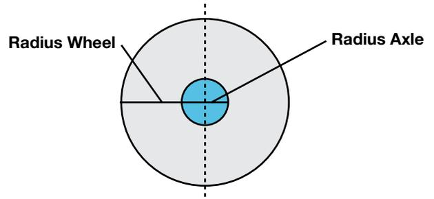
$$\text{Wheel and Axle MA} = \frac{\text{Radius of the wheel}}{\text{Radius of the axle}}$$
