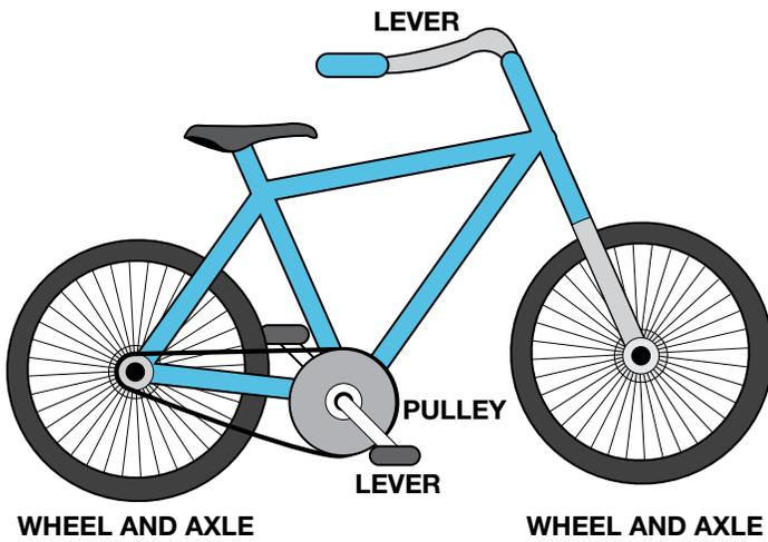
Most compound machines, especially in the transportation industry, are far more complex than bicycles or wheelbarrows. Planes, trains, cars, and trucks are compound machines built from thousands or tens of thousands of individual components, many of which are simple machines.
