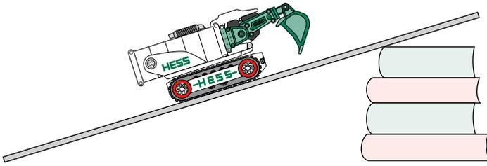
the loaded arm upward at different angles to test its effect on the Loader's balance.
