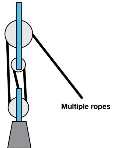
$$\text{Pulley MA} = \text{Number of ropes supporting the load}$$
