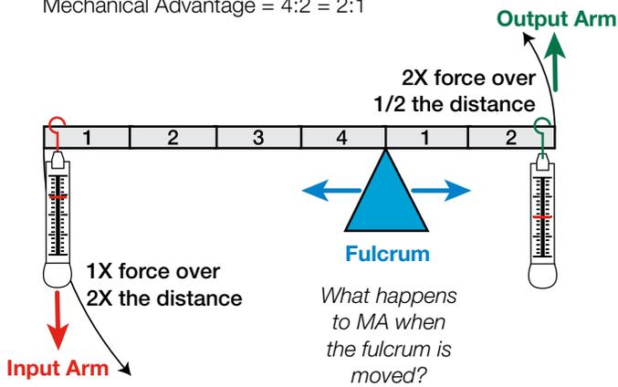
The mechanical advantage of a lever equals the length of the force input arm divided by the length of the output arm. In this example the MA is 2:1 or 2. To measure the forces with the spring scales, one student pulls down on the scale attached to the input arm while another student holds the scale attached to the output arm. Reading the scales reveals the mechanical advantage of the lever.
