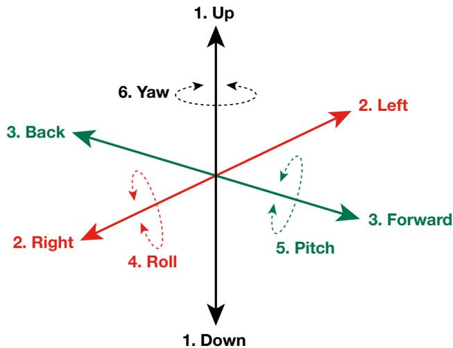
move in more than six different directions: (1) up/down, (2) right/left, (3) forward/back, and the rotating motions of (4) roll, (5) pitch and (6) yaw. Each movement is a degree of freedom. If a joint on a robot arm can move up and down, swing side to side, and rotate, the joint is said to have three degrees of freedom.
