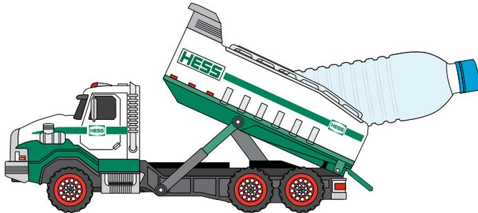
Have students try again with the bottle centered over the last “S” in the HESS name. Ask, *Can the truck dump the bottle now?* Follow with, *Why is the truck able to dump its load when the bottle is placed over the last “S” but not when the load is over the “H”?* (Remind students of mechanical advantage in levers. Moving the weight nearer to the fulcrum magnifies the lifting force.)
