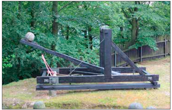
Twisted ropes (torsion) provided power to onager catapults, which threw heavy boulders against city or castle walls. Shown above is an onager catapult at Neurathen Castle in Germany.
