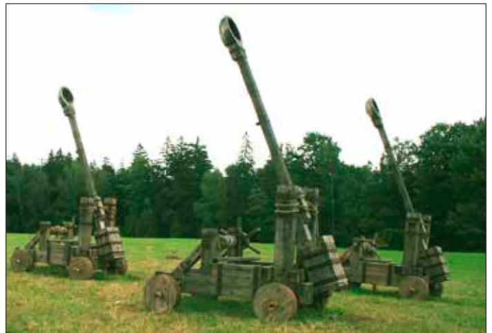
Medieval mobile onager catapults, each with a fixed bowl on an arm, were capable of hurling several projectiles at one time. The onagers shown above are in front of fortress Cuknštejn in South Bohemia, Czech Republic.
